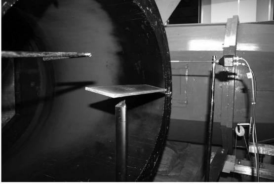
Fig. 4 Model set in the low-speed wind tunnel.
